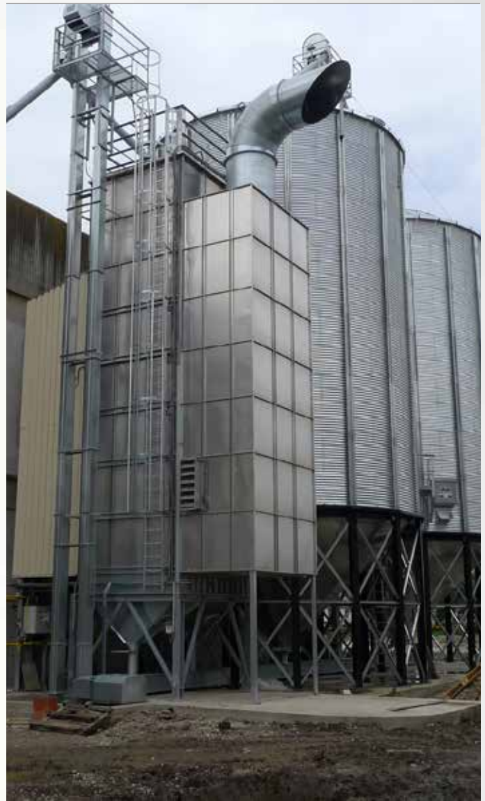
Project: Ostrov Czech Republic Type: GDB-XN 1/6-S Year: 2009 Product: maize, wheat Drying capacity: wheat: approx. 28,9 t/h from 19% to 15% maize: approx. 7,2 t/h from 35% to 15%
