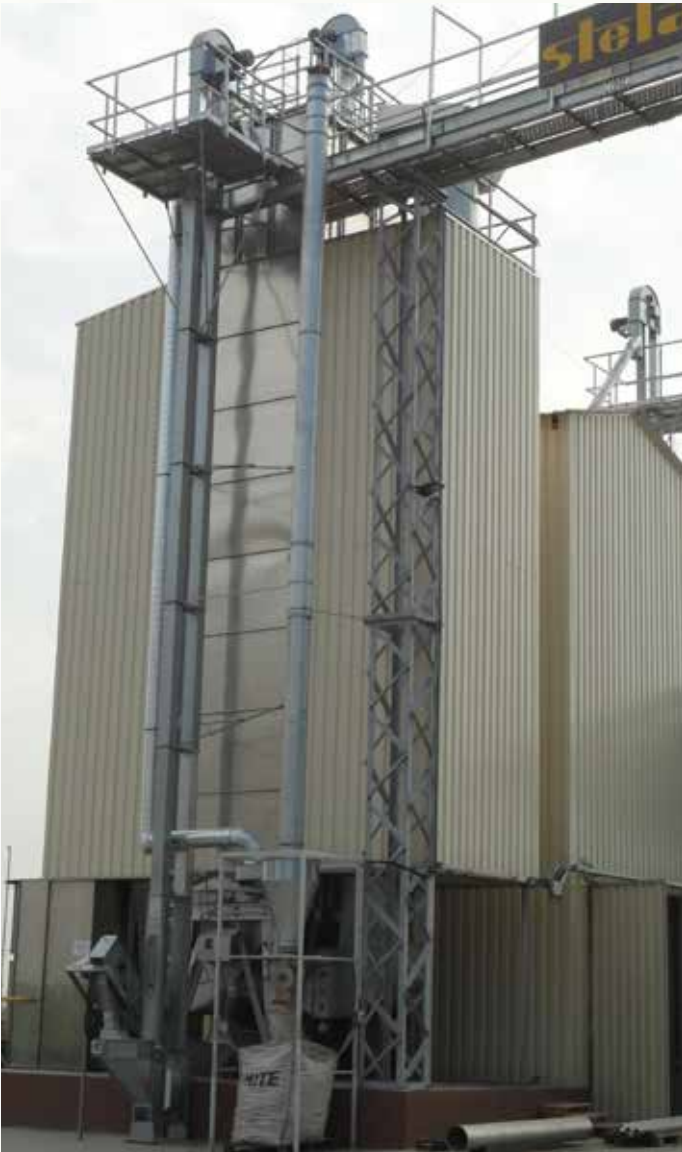
Project: Hevizgyörk Hungary Type: MDB-TN 1/8-SU Year: 2011 Product: maize Drying capacity: approx. 10,0 t/h from 25% to 15%
