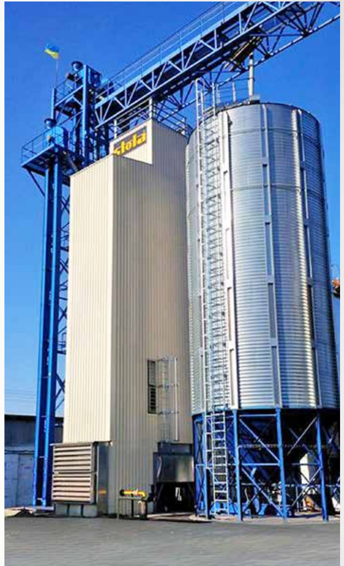
Project: Joint Stock Company Ukraine, Kremyn Type: MDB-XN 1/10-SU Year: 2013 Product: maize, wheat Drying capacity: wheat: ca. 38,5 t/h from 19% to 15% maize: ca. 14,0 t/h from 30% to 15%
