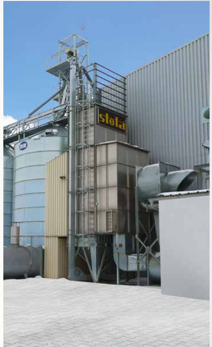
Project: Hostoun Czech Republic Type: GDB-TN 1/4-S Year: 2009 Product: maize Drying capacity: approx. 13,8 t/h from 19% to 15%
