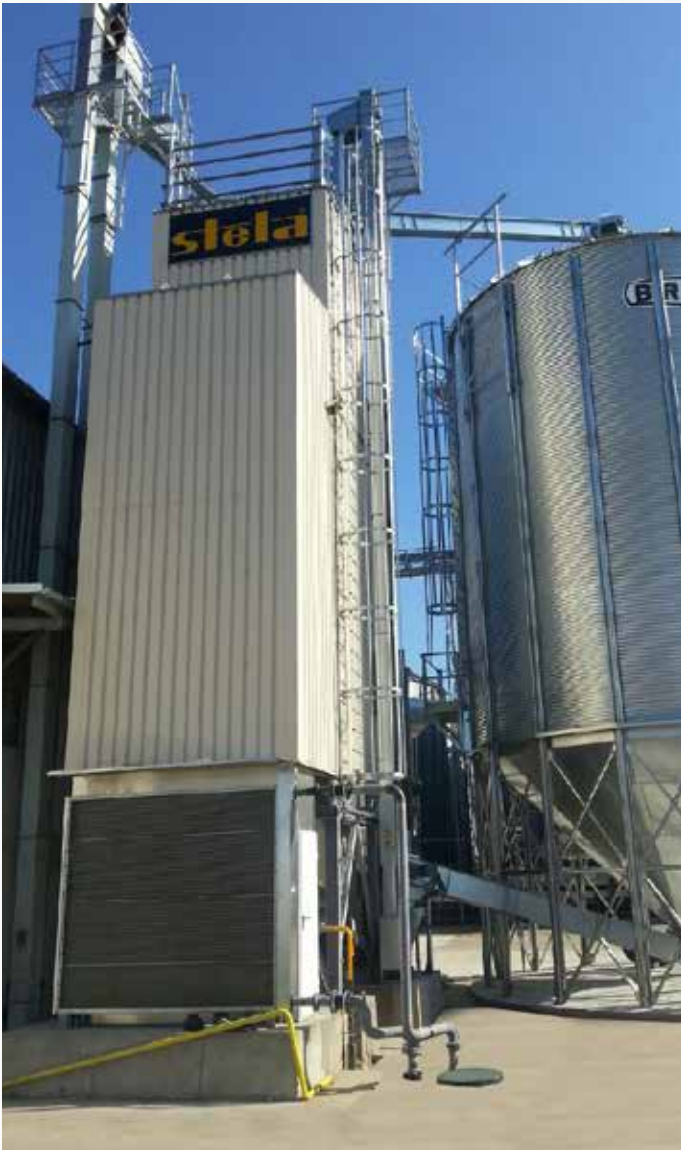
Project: Blazovice Czech Republic Type: MDB-XN 1/6-S Year: 2013 Product: maize Drying capacity: Mais: approx. 7,2 t/h from 35% to 15%
