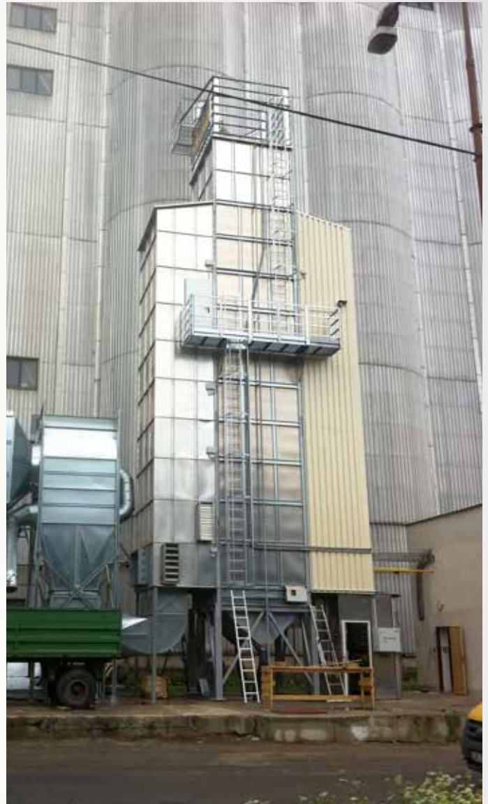
Project: Agrofert - Sedlcany Czech Republic Type: GDB-XN 1/10-S Year: 2011 Product: rapeseed Drying capacity: approx. 27,5 t/h from 12% to 8%
