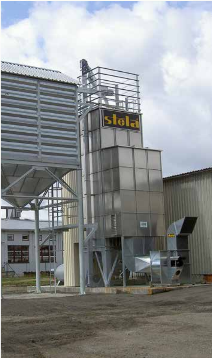
Project: Munice Czech Republic Type: MDB-TN 1/4-S Year: 2009 Product: maize Drying capacity: approx. 3,4 t/h from 35% to 15%
